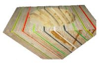
MDF ring over the top of the bowl. This will be turned away as late as possible. Wearing a glove to protect his hand, Dennis hollows the inside first using a Simon Hope tungsten carbide tipped tool. He uses a circle template to get the perfect round shape on the inside. This is indicated by a "bullseye" in the plywood rings.
