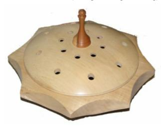
mounted the lid on the recess and proceeded to turn the top of the lid into a gentle curve. Using a homemade sanding drum, Alan sanded the holes. He also used a cotton bud to seal and wax them.
