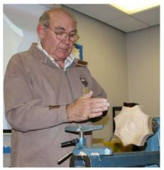
sanding sealer (thinned 50/50) and finished with Briwax applied with 0000 wire wool. This was buffed up using a soft cloth.
