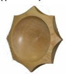
hollowed out the centre, re-sharpening his gouge before the last cut. He then power sanded to 320 grit for a better finish for the inside. Two coats of sanding sealer and Briwax
