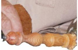
He then sanded 120 grit to 400 grit before sealing and waxing as before. After aligning the grain direction, the spigots were inserted into the holes in the plates. The top spigot only needed one spigot, with a ball on the
