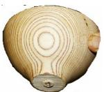
The outside of the bowl is turned in a similar manner, using bowl gouges, negative rake scrapers and TCT tools. Again, the aim is to get a second bullseye on the outside, before applying a super glue finish.
