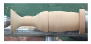
flowing cove from the top to nearly halfway down the 8" blank, leaving a thin (almost too thin) neck. As the neck opened out again into the body, Peter undercut and tapered the rest of the body slightly narrower than the top. He dished the top before sanding, sealing and waxing the bud vase. The plastic tube can be cut with a hacksaw if it is too long for the hole. After parting off, Peter sanded the bottom.
