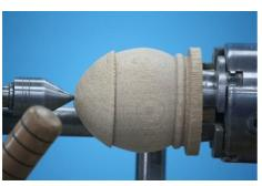
the chuck, Peter measured the opening in the base and transferred the measurement to the lid. He used a parting tool to cut a spigot on the lid that was a snug fit into the base. Peter hollowed the lid rather than leave it flat. After mounting the base back in the chuck, he fitted the lid and held it in place with the tail
