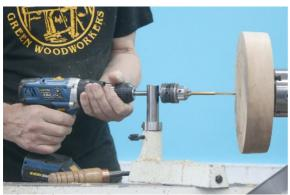
at 180° to the first. He then used a square to mark the third hole at 90° and the ruler again to mark the position of the fourth hole. After drilling all four leg holes, Phil cut a chucking recess on the underside of the seat. To do this, he used a beading/skew tool and also
