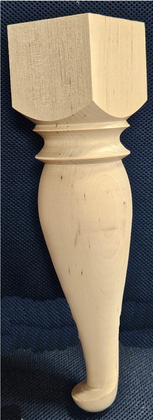
The finished Alan Batty style cabriole leg.
